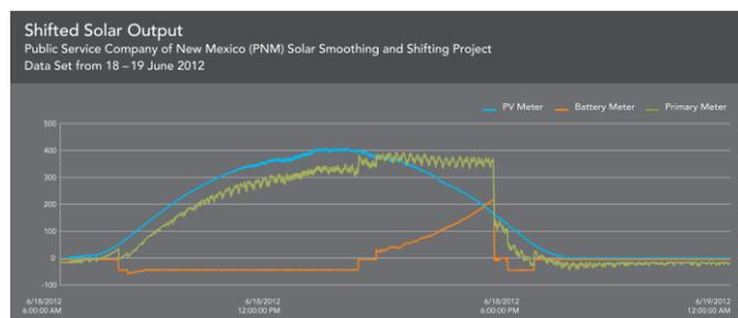
Fig. 6. Shifted Solar Output: UltraBattery® Solar Shifting Functionality Proven
