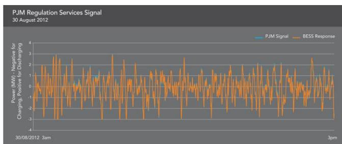
Fig. 8. Frequency Regulation: PJM Regulation Services Signal and Response of UltraBattery® Energy Storage System
