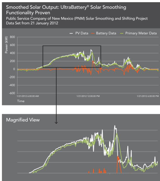
Fig. 7. Smoothed Solar Output: UltraBattery® Solar Smoothing Functionality Proven
