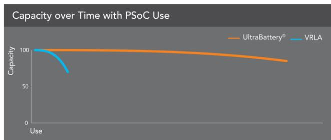
Fig. 3. Capacity over Time with Partial State of Charge (PSoC) Use
