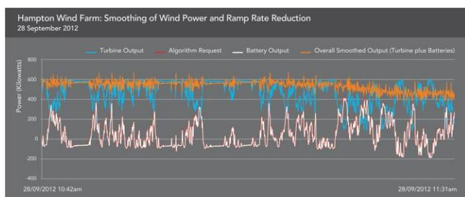
Fig. 4. Hampton Wind Farm: Smoothing of Wind Power and Ramp Rate Reduction
